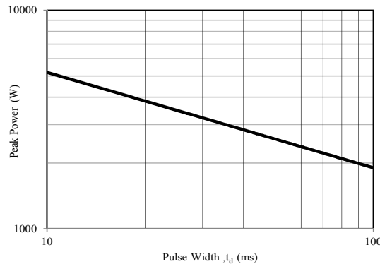
Fig. 4 - Peak Pulse Power Rating Curve
