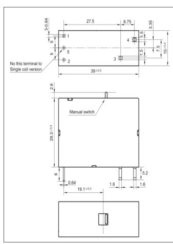
If no tolerance is shown: outline dimension <= 1mm, tolerance is  $\pm 0.2$ mm; outline dimension > 1mm and <=5mm, tolerance is  $\pm 0.3$ mm; outline dimension >5mm, tolerance is  $\pm 0.4$ mm.
