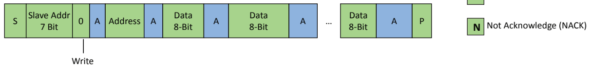
Register Block Write (I 2 C™ Write)
