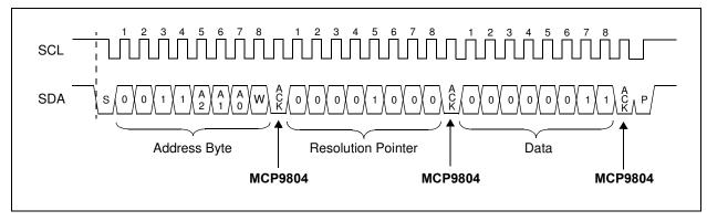
**FIGURE 5-8:** Timing Diagram for Changing  $T_A$  Resolution to  $+0.0625^{\circ}C$  <0000 0011>b (see Section 4.0 "Serial Communication").
