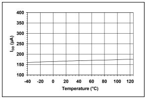
FIGURE 2-7: Supply Current vs. Temperature.
