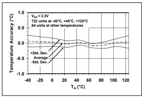
FIGURE 2-1: Temperature Accuracy.
