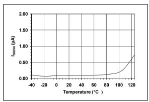
**FIGURE 2-8:** Shutdown Current vs. Temperature.
