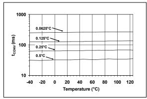
**FIGURE 2-12:** Temperature Conversion Time vs. Temperature.
