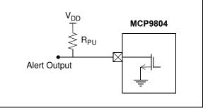
FIGURE 5-9: Active-Low Alert Output Configuration.
