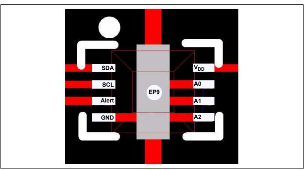
FIGURE 6-1: DFN Package Layout (Top View).
