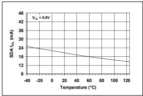
FIGURE 2-14: SDA I<sub>OL</sub> vs. Temperature.
