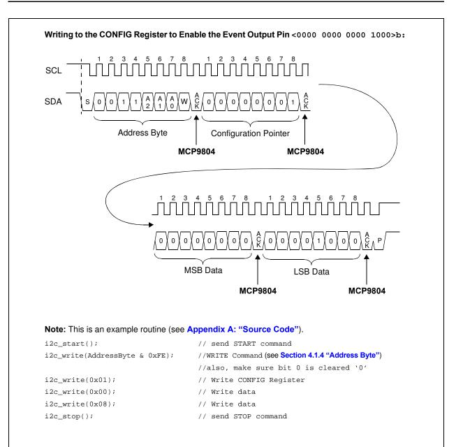
**FIGURE 5-2:** Timing Diagram for Writing to the Configuration Register (see **Section 4.0 "Serial Communication"**).
