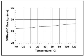
FIGURE 2-16: SMBus Time-out vs. Temperature.
