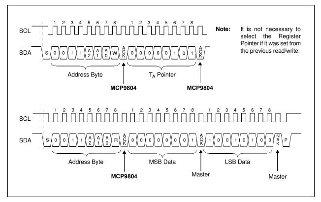
**FIGURE 5-5:** Timing Diagram for Reading  $+25.25^{\circ}C$  Temperature from the  $T_A$  Register (see Section 4.0 "Serial Communication").
