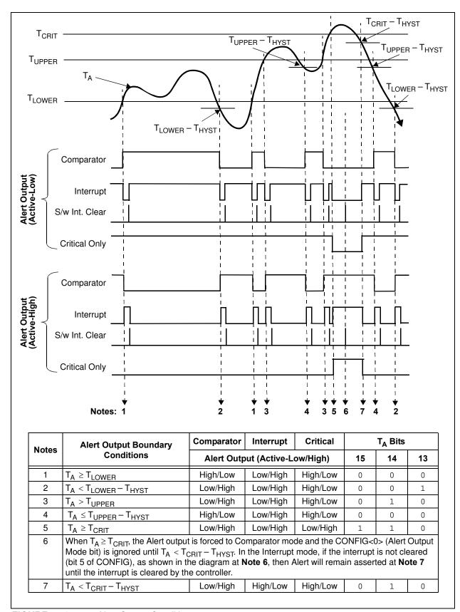
FIGURE 5-10: Alert Output Conditions.
