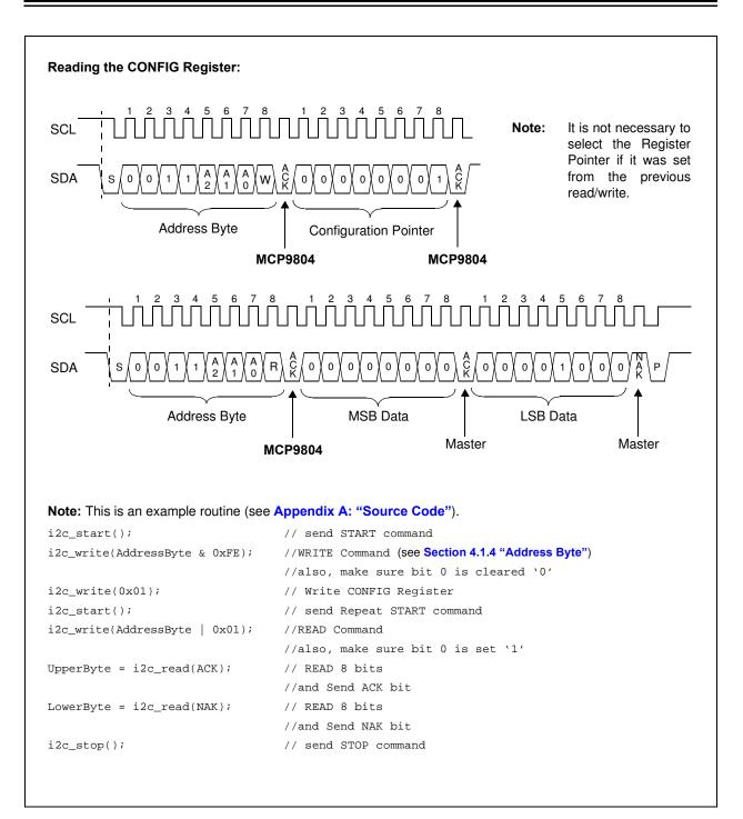
**FIGURE 5-3:** Timing Diagram for Reading from the Configuration Register (see **Section 4.0 "Serial Communication"**).
