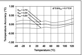
**FIGURE 2-10:** Temperature Accuracy vs. Supply Voltage.
