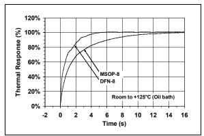
**FIGURE 2-15:** Package Thermal Response.
