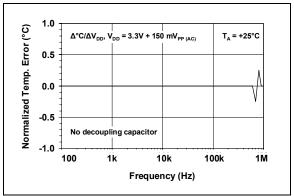
**FIGURE 2-11:** Power Supply Rejection vs. Frequency.
