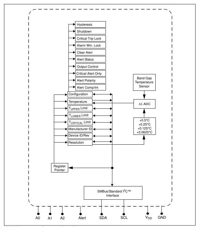
FIGURE 5-1: Functional Block Diagram.
