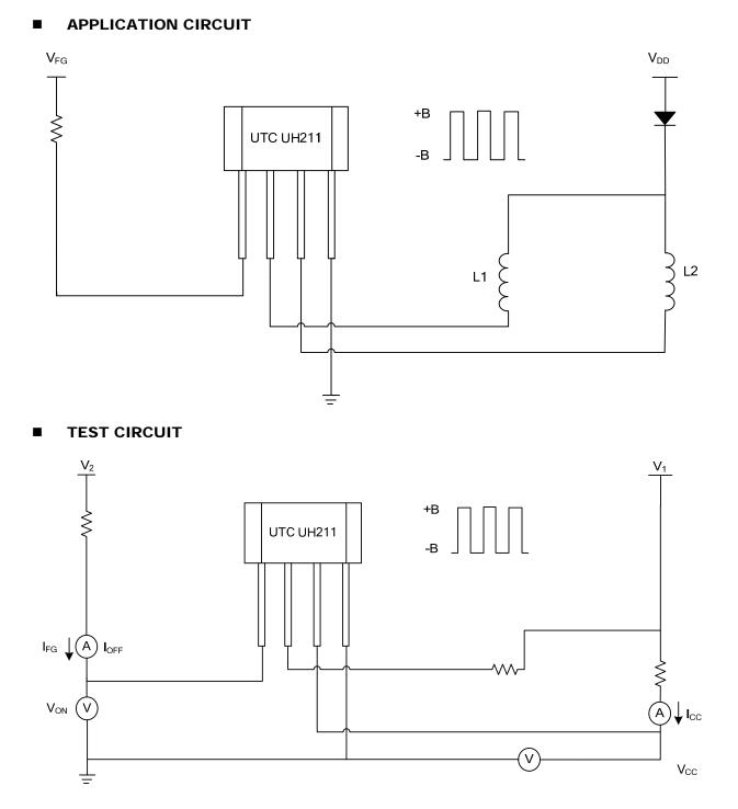
Measure  $V_{\text{CC}},I_{\text{CC}}$  when DO is off. Measure  $V_{\text{ON}},I_{\text{FG}}$  when FG is on. Measure  $I_{\text{OFF}}$  when FG is off.
