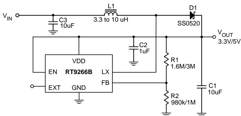
Figure 1. RT9266B Typical Application for Portable Instruments
