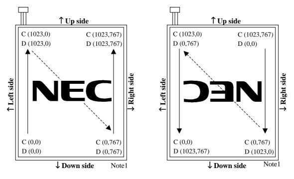
Figure 1. Normal scan (DPSR: Low or Open)
