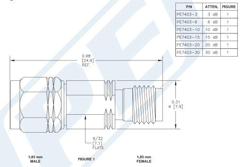
20 dB Fixed Attenuator, 1.85mm Male To 1.85mm Female Passivated Stainless Steel Body Rated To 1 Watt Up To 65 GHz from Pasternack Enterprises has same day shipment for domestic and International orders. Our RF, microwave and millimeter wave products maintain a 99% availability and are part of the broadest selection in the industry.
