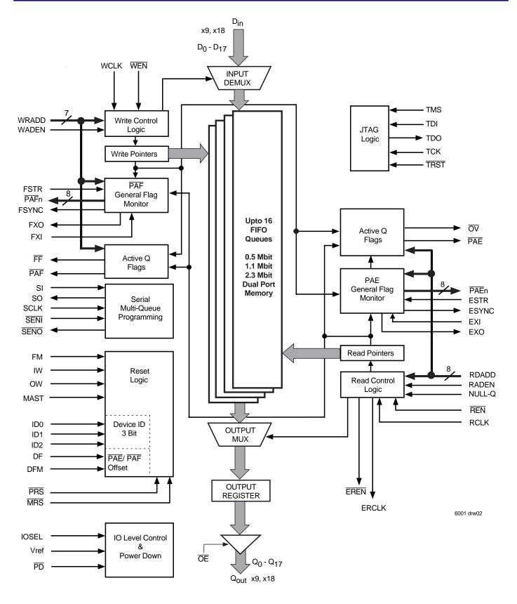
Figure 1. Multi-Queue Block Diagram
