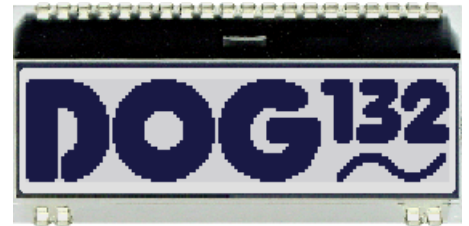
Orientation for 6 o'clock (Bottom View)
