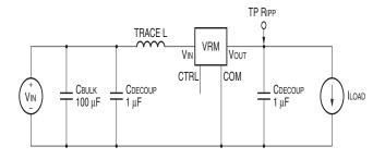
Figure 44. Input /Output Decoupling Circuit.
