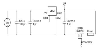
Figure 45. Load Transient Circuit.
