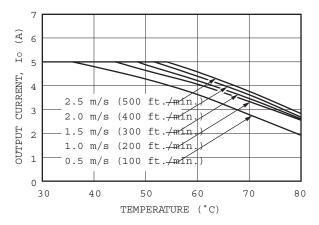
Figure 41. Thermal Derating for 5.0VIN ,2.0VOUT.
