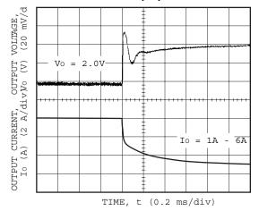
Figure 27. Transient Response Characteristic of 3.3VIN/2.0VOUT with IOUT step up 6A-1A Static load.
