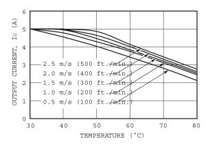
Figure 40. Thermal Derating for 5.0VIN ,1.8VOUT.
