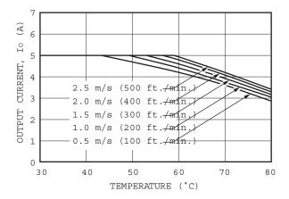
Figure 38. Thermal Derating for 3.3VIN ,2.0VOUT.
