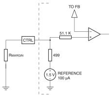
Figure 47. Circuit for decreasing the output voltage.
