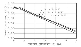
Figure 21. Stactic Regulation: 5.0VIN,3.3VOUT.
