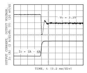
Figure 34. Transient Response Characteristic of 5.0VIN/ 3.3VOUT with IOUT step up 1A-6A Static load.
