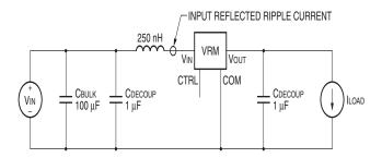
Figure 43. Input Reflected Ripple Current Test Setup.
