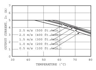
Figure 39. Thermal Derating for 3.3VIN ,2.5VOUT.
