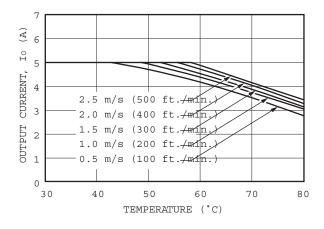
Figure 37. Thermal Derating for 3.3VIN ,1.8VOUT.
