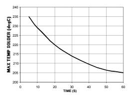
Figure 51. Time Limit curve above 205<sup>0</sup>C.
