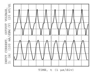
Figure 8. Typical Ripple Performance with 6.2A resistive load at 3.3VIN,1.5VOUT.
