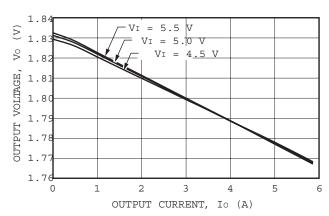
Figure 16. Static Regulation 3.3VIN.1.8VOUT.
