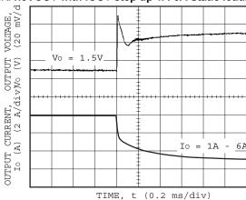
Figure 23. Transient Response Characteristic of 3.3VIN/1.5VOUT with IOUT step up 6A-1A Static load.
