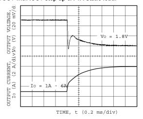
Figure 30. Transient Response Characteristic of 5.0VIN/ 1.8VOUT with IOUT step up 1A-6A Static load.
