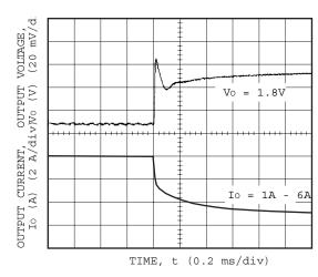
Figure 31. Transient Response Characteristic of 5.0VIN/ 1.8VOUT with IOUT step up 6A-1A Static load.
