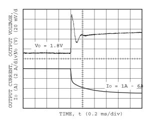
Figure 25. Transient Response Characteristic of 3.3VIN/1.8VOUT with IOUT step up 6A-1A Static load.
