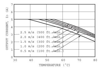
Figure 42. Thermal Derating for 5.0VIN ,3.3VOUT.
