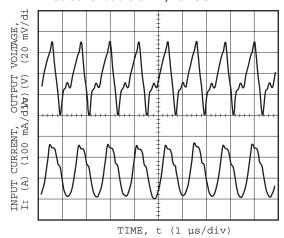
Figure 10. Typical Ripple Performance with 6.2 A resistive load 3.3VIN,2.0VOUT.
