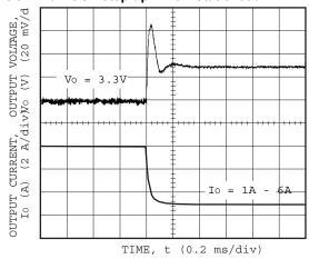
Figure 35. Transient Response Characteristic of 5.0VIN/ 3.3VOUT with IOUT step up 6A-1A Static load.
