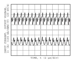
Figure 11. Typical Ripple Performance with 6.2A resistive load 3.3VIN,2.5VOUT.
