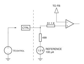
Figure 46. Circuit for increasing the output voltage.
