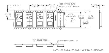
Note: Austin Lite Power Modules are shipped in quantities of 250 modules per tape and reel.
