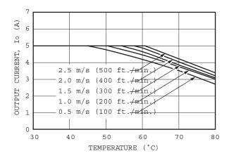
Figure 36. Thermal Derating for 3.3VIN ,1.5VOUT.
