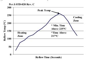
Figure 52. Recommended linear reflow profile using Sn/Ag/Cu solder.
