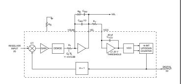
FIGURE 2. TRANSFER FUNCTION BLOCK DIAGRAM #1
