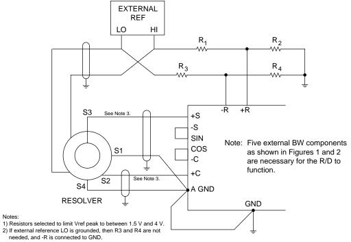
3) 10k ohms, 1 % series current limit resistors are recommended.
