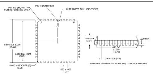
FIGURE 17. RDC-19222S (44-PIN PLASTIC J-LEAD) MECHANICAL OUTLINE
