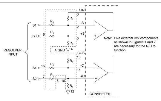
S1 and S3, S2 and S4, and RH and RL should be ideally twisted shielded, with the shield tied to AGND at the converter.
