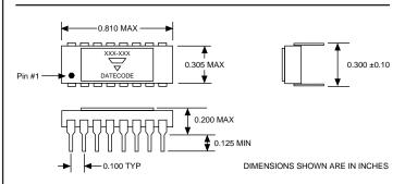
FIGURE 23. 16-PIN THIN-FILM RESISTOR NETWORK DIP MECHANICAL OUTLINE - CERAMIC PACKAGE (DDC-49590)
