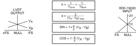
FIGURE 12B. 3-WIRE LVDT SCALING CIRCUIT
