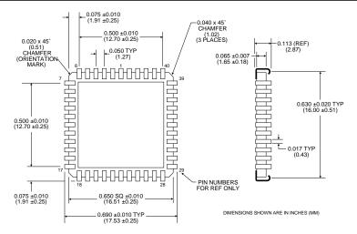
FIGURE 18. RDC-19222S (44-PIN CERAMIC J-LEAD) MECHANICAL OUTLINE
