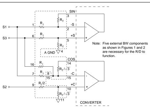
S1, S2, and S3 should be triple twisted shielded; RH and RL should be twisted shielded, In both cases the shield should be tied to AGND at the converter. 90 V input = DDC-49590: Ri = 270 k $\Omega$ , 90 V input, synchro or resolver. 11.8 V input = DDC-49530: Ri = 70.8 k $\Omega$ , 11.8 V input, synchro or resolver. Maximum addition error is 1 LSB.
