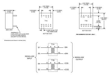
FIGURE 6B. TRANSFORMER LAYOUT AND SCHEMATIC (RESOLVER INPUT - 52036/52037/52038)
