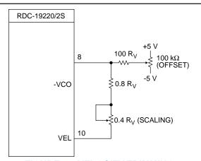
FIGURE 11. VELOCITY TRIMMING
