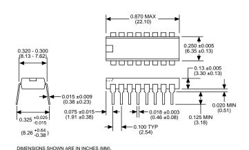
FIGURE 21. 16-PIN THIN-FILM RESISTOR NETWORK DIP MECHANICAL OUTLINE (DDC-49530, DDC-55688-1)
