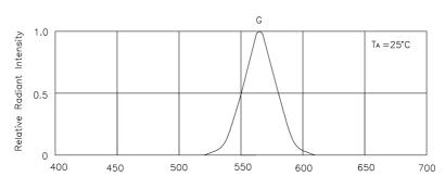
wavelength  $\lambda$  (nm) RELATIVE INTENSITY Vs. WAVELENGTH
