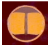
Elcon uses eye of the needle compliant press-fit tails for optimum interface to the board.
