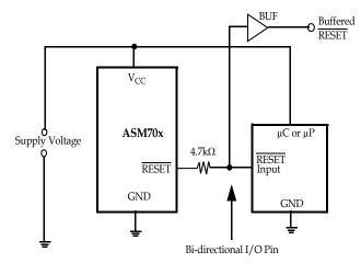
Figure 3: Bi-directional reset pin interfacing
