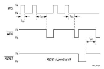
Figure 1: WDI Three-state operation
