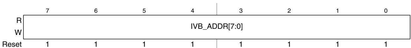
Figure 7-2. Interrupt Vector Base Register (IVBR)
