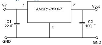
C1: A low ESR capacitor is required to keep the converter to a minimum. Ceramic capacitors are recommended, but tantalum or electrolytic may be used. Typical value is 22µF / 50V.
