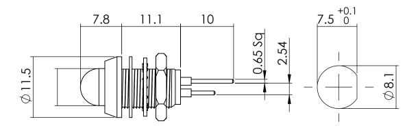
Dimensions in mm (typical) Not to scale Anode termination denoted by red indicator Mounting hole to be clean and burr free
