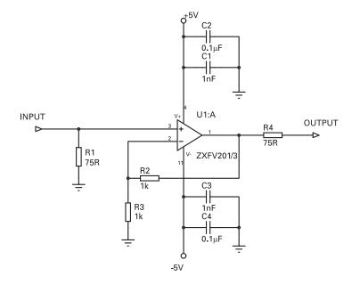
Figure 1: Typical video signal application circuit, gain = 2 (overall gain = 1 for 75 $\Omega$  load)
