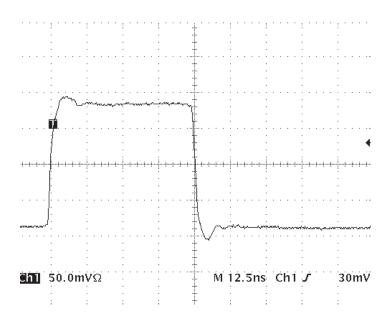
Figure 2: Pulse response, unity gain, 1V\_{PP}, R\_F = 510 $\Omega$
