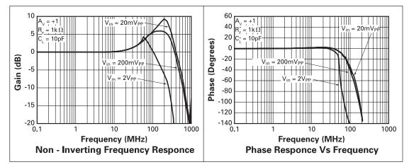
Figure 3: Graphs of gain and phase vs frequncy ( $R_1 = 150\Omega$ )
