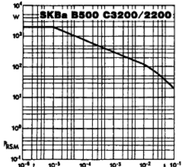
Fig. 7 Rated reverse power dissipation vs. time
