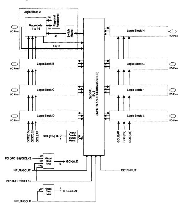
The ATF1508 macrocell is flexible enough to support highly complex logic functions operating at high speed. The macrocell consists of five sections: product terms and product term select multiplexer; OR/XOR/CASCADE logic; a flip-flop; output select and enable; and logic array inputs.
