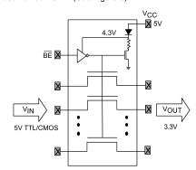
FIGURE 3. Fairchild Semiconductor's FSTD device incorporating the diode translation function and a switch to eliminate current flow during High Impedance mode.
