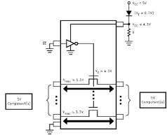
FIGURE 2. Typical 5V to 3V Translation Circuit
