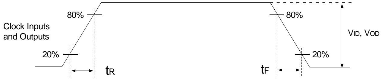
Figure 8. Input and Output Slew Rates
