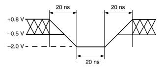
Figure 10. Maximum Negative Overshoot Waveform
