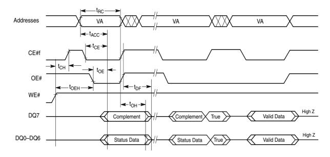
**Notes:**Note: VA = Valid address. Illustration shows first status cycle after command sequence, last status read cycle, and array data read cycle.
