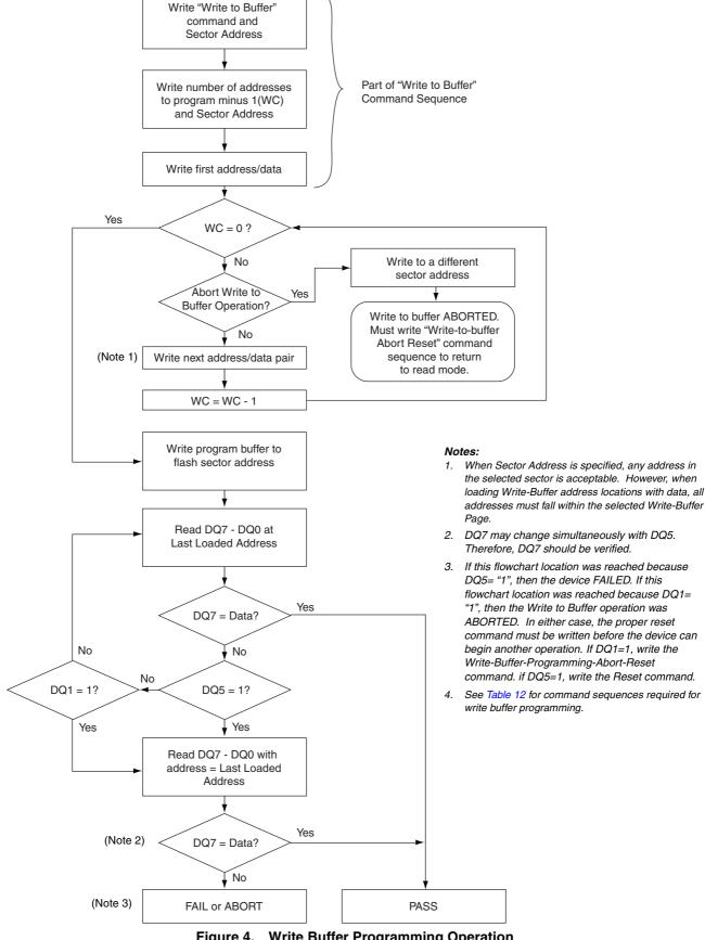
Figure 4. Write Buffer Programming Operation
