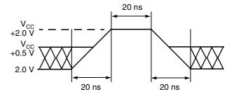
Figure 11. Maximum Positive Overshoot Waveform
