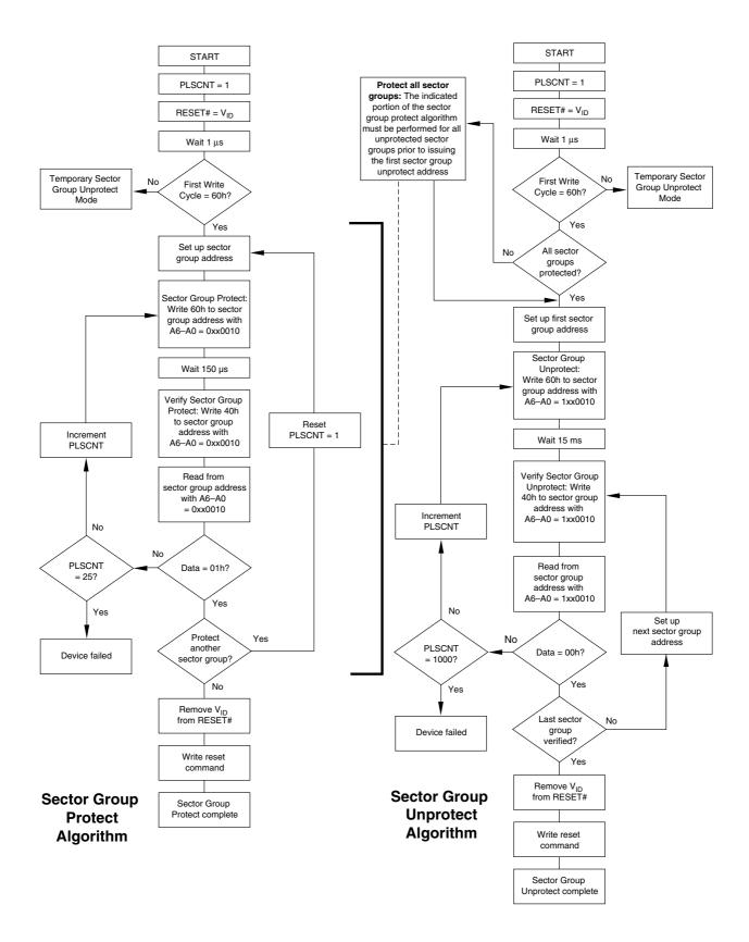
Figure 2. In-System Sector Group Protect/Unprotect Algorithms
