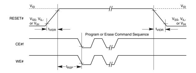
Figure 23. Temporary Sector Group Unprotect Timing Diagram
