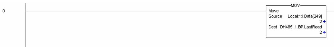
The module will send block identification code 0 (and possibly -1 if not configured for any read blocks) to the processor. These blocks will only contain the status data. The following rung shown displays logic to handle these blocks:
