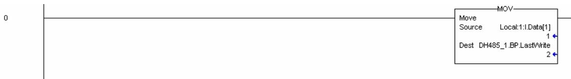
The next two rungs are used to handle processor control of the module using the warm- and cold- boot control block numbers. When the processor requires the module to perform one of these operations, it simply copies the block number into the output image of the module and the module will perform the operation. Be certain to set the required block number in the last write object to prevent further processing in the WriteData task. Examples of each control block is given below:
