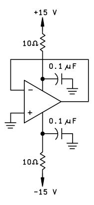
FIGURE 2. Radiation exposure circuit.
