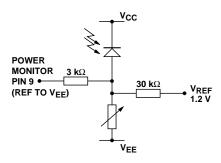
Figure 2b. Power Monitor Circuit.
