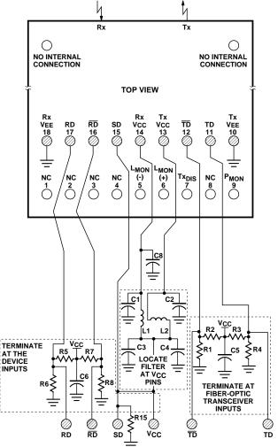
NOTES: — THE SPLIT-LOAD TERMINATIONS FOR PECL SIGNALS NEED TO BE LOCATED AT THE INPUT OF DEVICES RECEIVING THOSE PECL SIGNALS. R1 = R4 = R6 = R8 = 130  $\Omega$ . R2 = R3 = R5 = R7 = 82  $\Omega$ . R15 = 10 K. C1 = C2 = C3 = C5 = C6 = 0.1  $\mu$ F.
