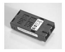
The new multisourced 2 x 9 footprint package style is a variation of the standard 1 x 9 package with an integral Duplex SC connector receptacle. The extra row of 9 pins provides connections for laser bias and optical power monitoring as well as providing transmitter disable function. A block diagram is shown in Figure 1.
