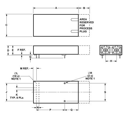
NOTE 1: SOLDER POSTS AND ELECTRICAL PINS ARE TIN/LEAD PLATED.
