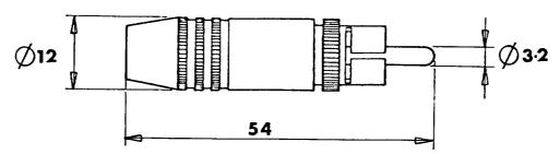
A range of high quality UK manufactured phono plugs made from machined brass with various plating options. The contact can be removed from the main body when crimping preference is preferred on assembling cable to contact.
