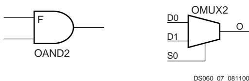
Figure 7: AND and MUX Symbols in Spartan-XL IOB
