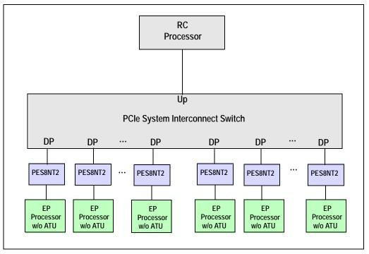
Figure 2 Embedded Compute Application - Processors With and Without Address Translation Unit (ATU) Functionality
