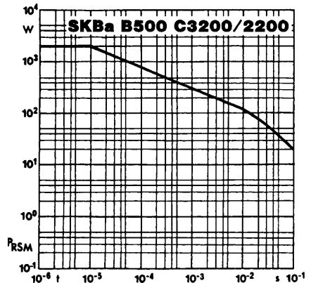
Fig. 7 Rated reverse power dissipation vs. time
