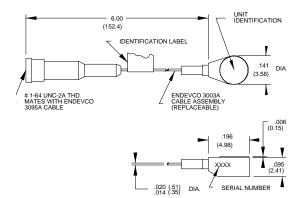
STANDARD TOLERANCE INCHES (MILLIMETERS) .XX = +/- .02 (.X = +/- .5) .XXX = +/- .010 (.XX = +/- .25)
