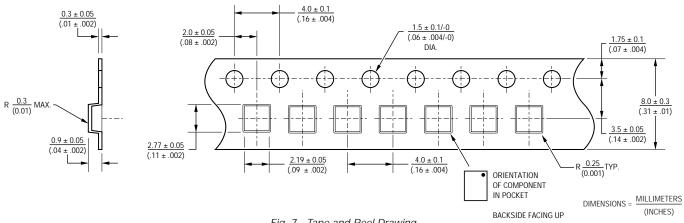
Fig. 7 - Tape and Reel Drawing
