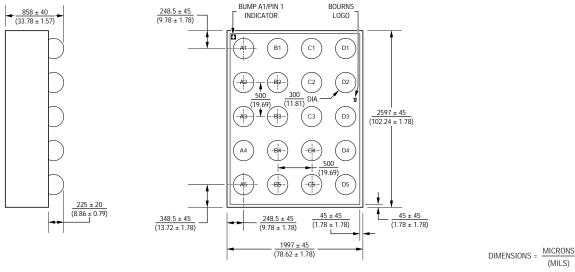
Fig. 2 – Device Mechanical Drawing
