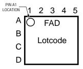
Fig. 5 – Backside Laser Mark
