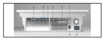
A: Line-in/Line-out/Mic-in B: USB 2.0 x 4
