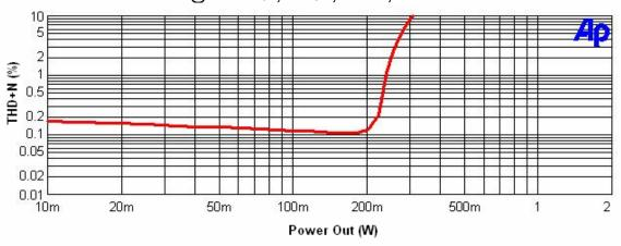
Figure 12 THD+N vs Power Out @ VDD=2.6V, RL=4Ω, f=1kHz, Av=2
