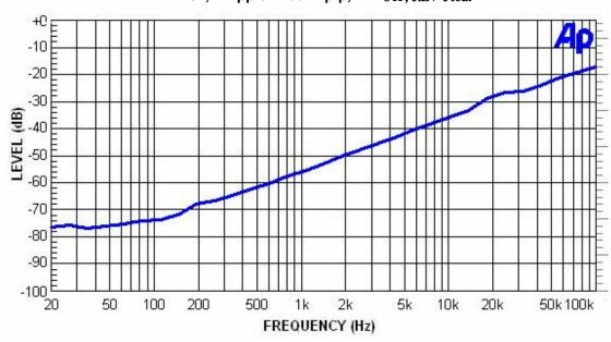
Figure 16 Power Supply Rejection Ratio (PSRR) @ Av=4 VDD=3V, V ripple =200mvp-p, RL= $8\Omega$ , RIN=Float
