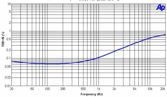
Figure 5 **THD+N vs Frequency** at VDD=3V, RL= $8\Omega$ , PWR=250mW, Av=2
