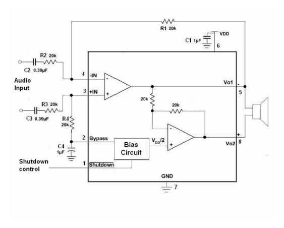
Figure 2. Audio Amplifier with Differential Input
