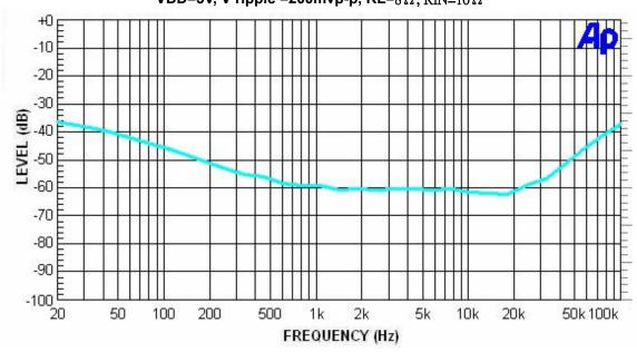
Figure 22 Power Supply Rejection Ratio (PSRR) @ Av=4 VDD=3V, V ripple =200mvp-p, RL= $8\Omega$ , RIN= $10\Omega$
