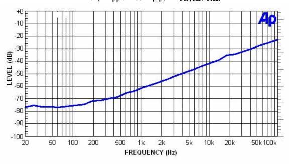
Figure 14 Power Supply Rejection Ratio (PSRR) @ Av=2 VDD=3V, V ripple =200mvp-p, RL= $8\Omega$ , RIN=Float
