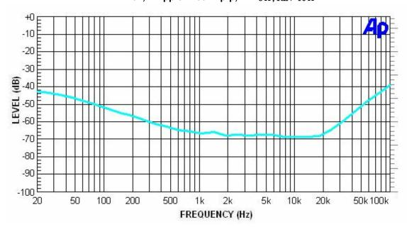
Figure 18 Power Supply Rejection Ratio (PSRR) @ Av=2 VDD=3V, V ripple =200mvp-p, RL= $8\Omega$ , RIN= $10\Omega$
