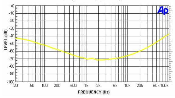
Figure 20 Power Supply Rejection Ratio (PSRR) @ Av=2 VDD=2.6V, V ripple =200mvp-p, RL= $8\Omega$ , RIN= $10\Omega$
