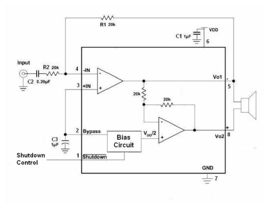
Figure 1. Audio Amplifier with Single -Ended Input
