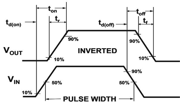
Figure 2:Switching Waveforms
