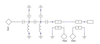
The internal configuration of the Ultra low profile filter balun is diagramed to the left. A lumped element filter is located in front of the unbalanced input of the balun. The unbalanced port is terminated in an open-circuit and the two balanced ports are connected to ground.
