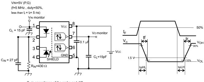
$C_L$  is capacitance of the probe and JIG. (P.G) : Pulse Generator
