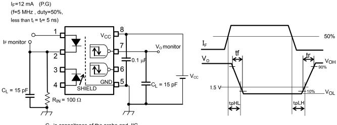
$C_L$  is capacitance of the probe and JIG. (P.G) : Pulse Generator
