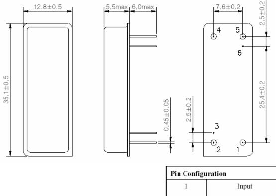
Pin Configuration1Input5Output2, 4GroundOtherCase ground
