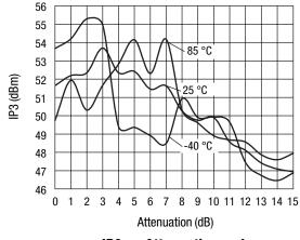
IP3 vs. Attenuation and Temperature (500 MHz)
