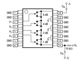
DC blocking capacitors (CBL) and biasing resistor must be supplied externally for positive voltage operation.
