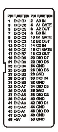
Table 1: Block Diagram and 50-Pin Connector Pin Assignments
