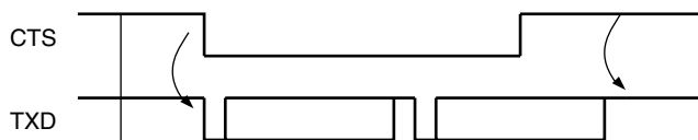
Figure 30-18. Transmitter Behavior when Operating with Hardware Handshaking
