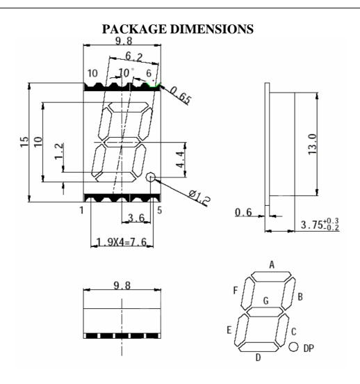
NOTES: All dimensions are in millimeters. Tolerances are  $\pm$  0.25-mm (0.01") unless otherwise noted. INTERNAL CIRCUIT DIAGRAM
