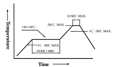
3. DIP soldering (Wave Soldering):
