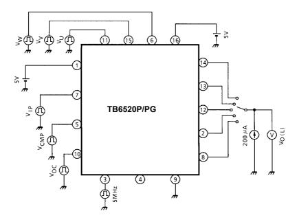
• Input amplitude 1.5 to 3.5 V to VU, VV, VW, VIP, VCMP, and VOC, and cause the output to function.
