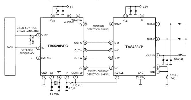
Note) Utmost care is necessary in the design of the output, V<sub>CC</sub>, V<sub>M</sub>, and GND lines since the IC may be destroyed by short-circuiting between outputs, air contamination faults, or faults due to improper grounding, or by short-circuiting between contiguous pins.
