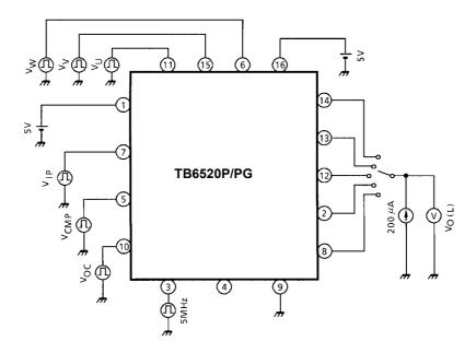
ullet Input amplitude 1.5 to 3.5 V to VU, VV, VW, VIP, VCMP, and VOC, and causes the output to function.
