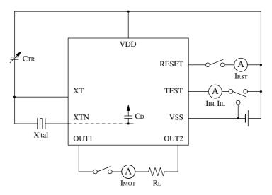
X' tal parameters: f = 32.768kHz, CI = 20k $\Omega$ , C0 = 1.3pF, C1 = 2.6fF
