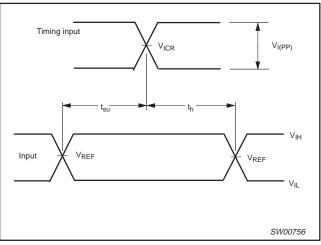
Waveform 5. Setup and hold times
