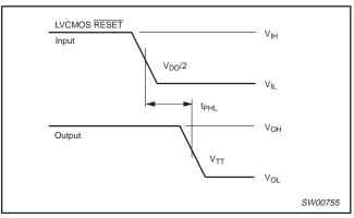
Waveform 4. Propagation delay times
