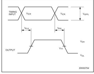
Waveform 3. Propagation delay times
