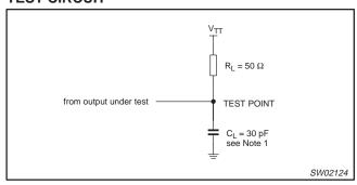
Figure 1. Load circuitry
