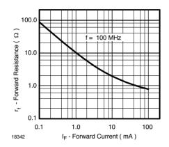
Fig. 1 Forward Resistance vs. Forward Current
