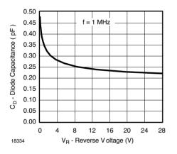
Fig. 2 Diode Capacitance vs. Reverse Voltage
