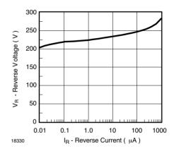
Fig. 4 Reverse Voltage vs. Reverse Current
