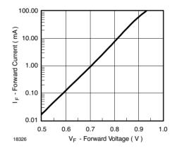
Fig. 3 Forward Current vs. Forward Voltage
