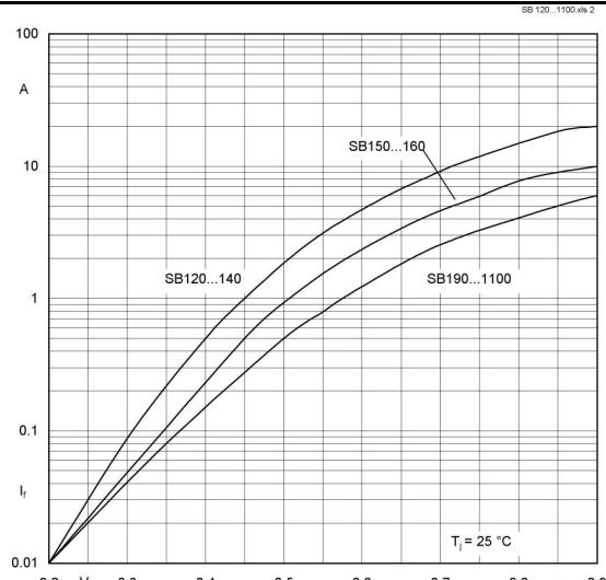
Fig. 1 Forward characteristics ( typical values )
