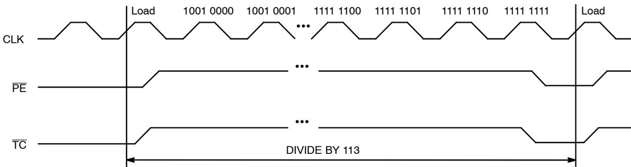
Figure 5. Divide by 113 EP016A Programmable Divider Waveforms
