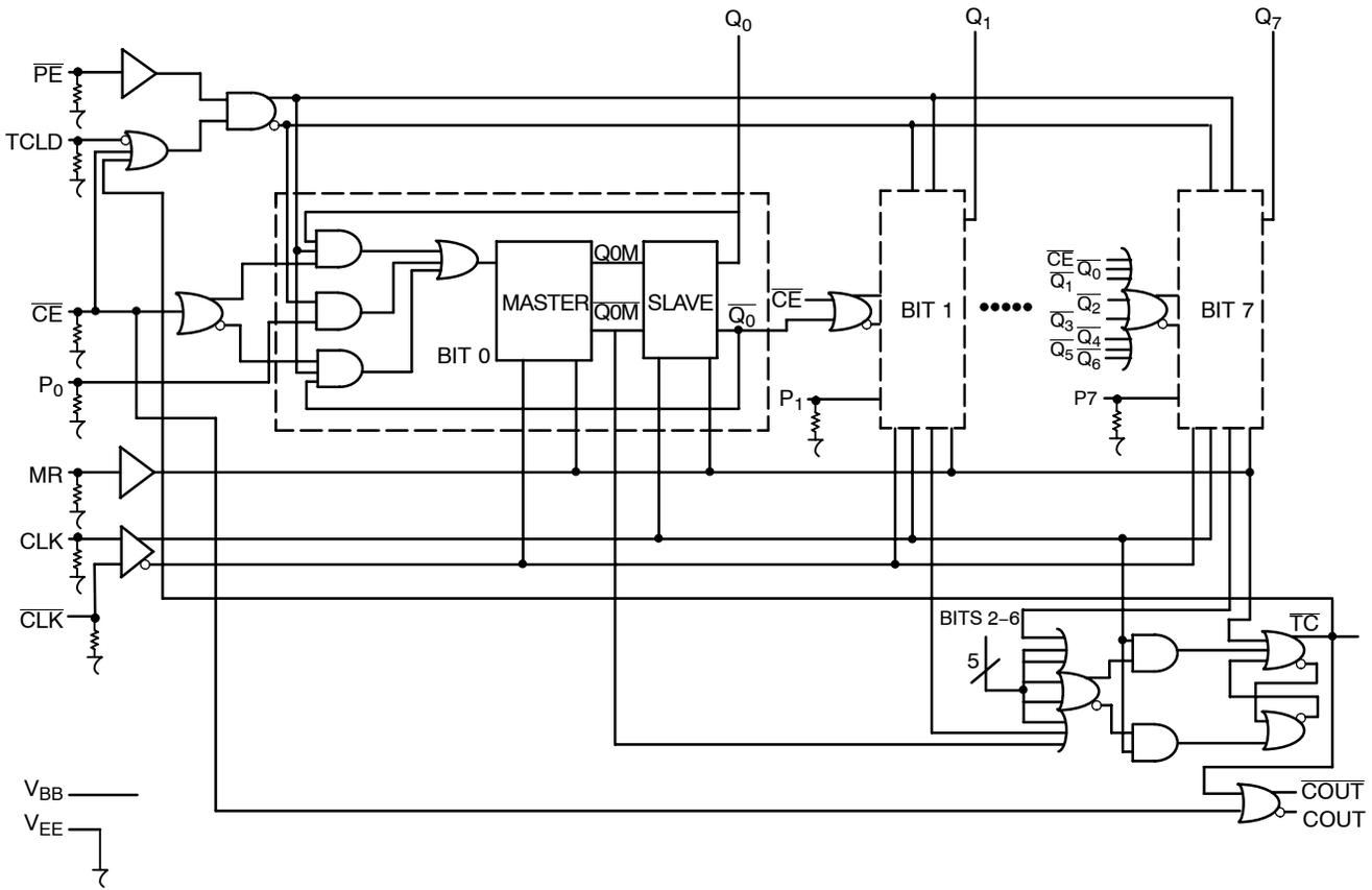
Note that this diagram is provided for understanding of logic operation only. It should not be used for propagation delays as many gate functions are achieved internally without incurring a full gate delay.
